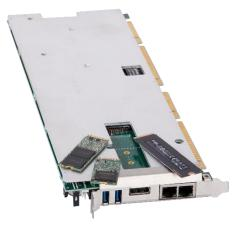
was required. Two emerging standards are competing to become the de facto physical standard in high-speed nonvolatile storage, M.2 and U.2. The Trenton TKL8255 is launching with provisions for M.2 drives, pictured right.
